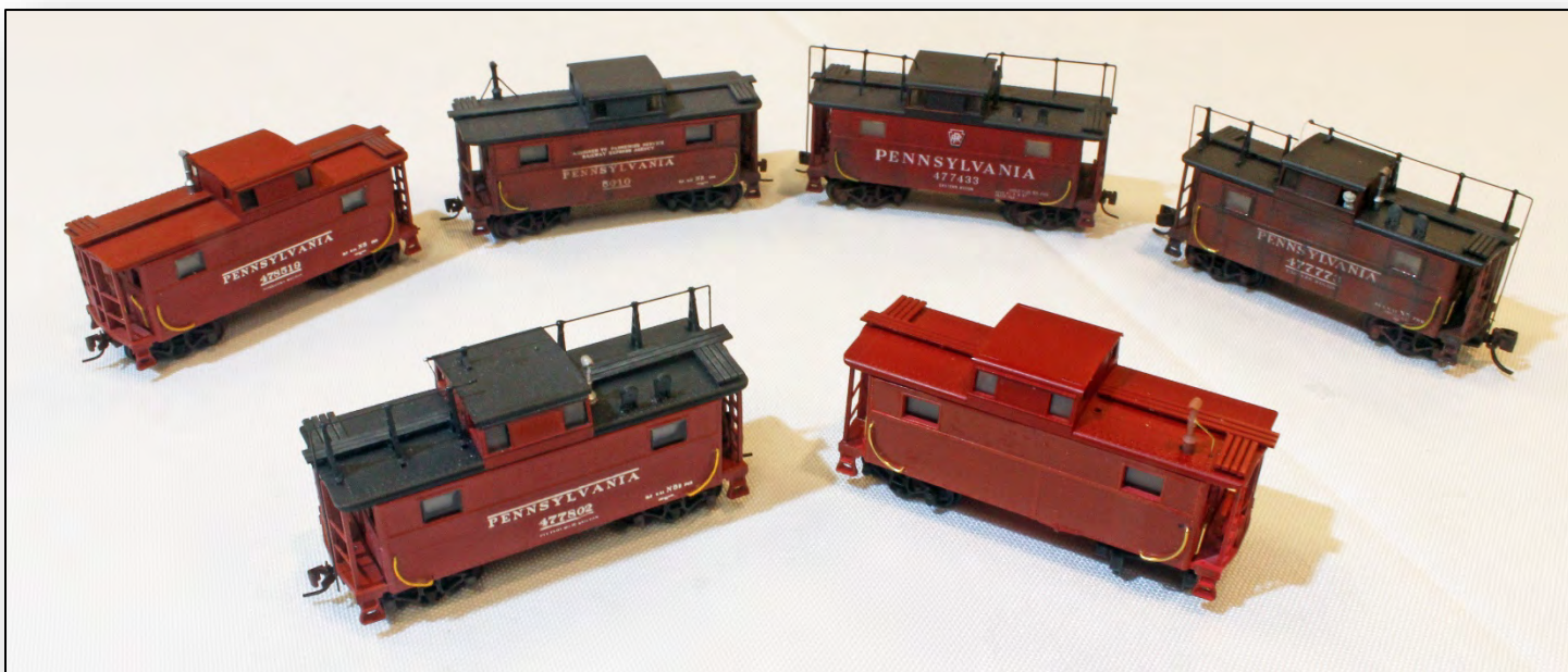
Doug Nelson assembled this collection of N-scale N5 and N5b cabin cars circa 1946-1953. They are kitbashed and detailed from Bowser N5 cars. Doug added grab irons, smoke jacks, and Trainphone antennas. Five different schemes are shown along with one car in progress.
