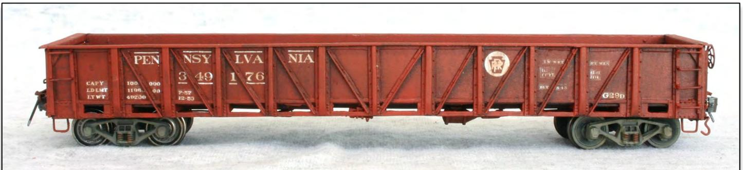
Figure 23. Model after weathering with acrylic paints.
