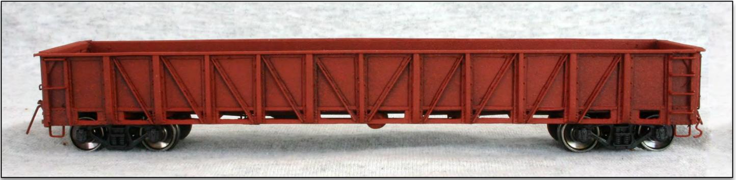
**Figures 18.** Model after application of PRR freight car color and trucks.
