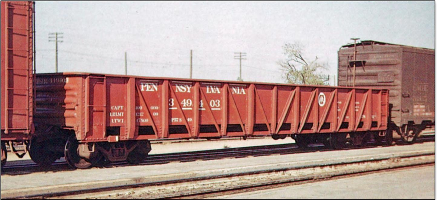
**Figure 2.** Prototype photo of G29D #349403 with the circle keystone lettering scheme taken in 1951. (Photo by K.B. King Jr from the Dick Kuelbs collection. Photo used with permission from the PRR Color Guide to Freight and Passenger Equipment, David R Sweetland and Robert J Yanosey, ©1992, Morning Sun Books, Inc.)
