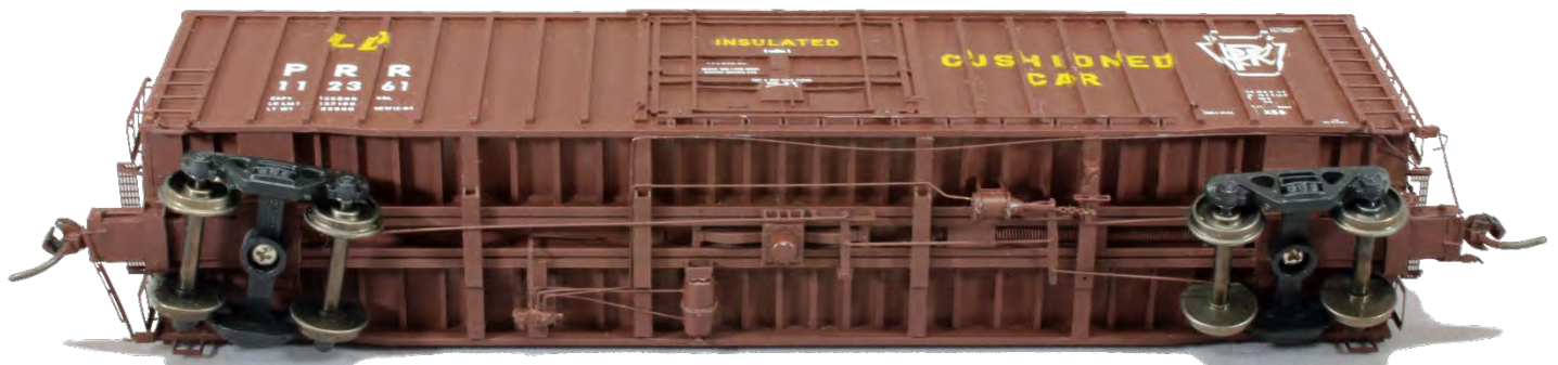
X58 boxcar with Hydra cushion underframe.
