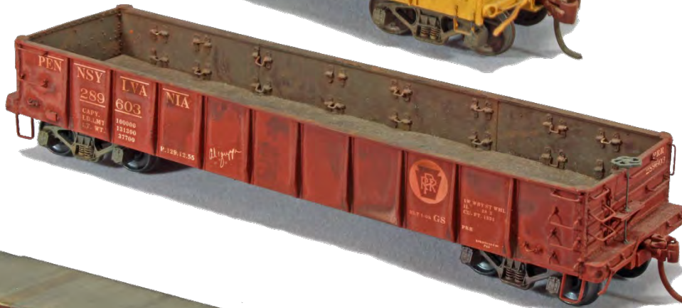
This GS gondola has a 5-spoke scalloped brake-wheel and interior folding stake pockets.
