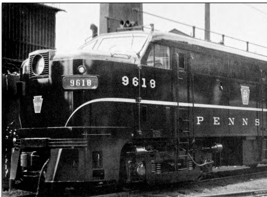
November 1951 builder's photos (here and top of next page) of 9818A shown with the coupler doors spread open and the pilot arch rotated up. In the down position it provided support for the bottom of the doors but would hit the arch on a unit coupled nose to nose if not rotated up (and back). Note placement of nose ladder rest grab irons at an angle.
