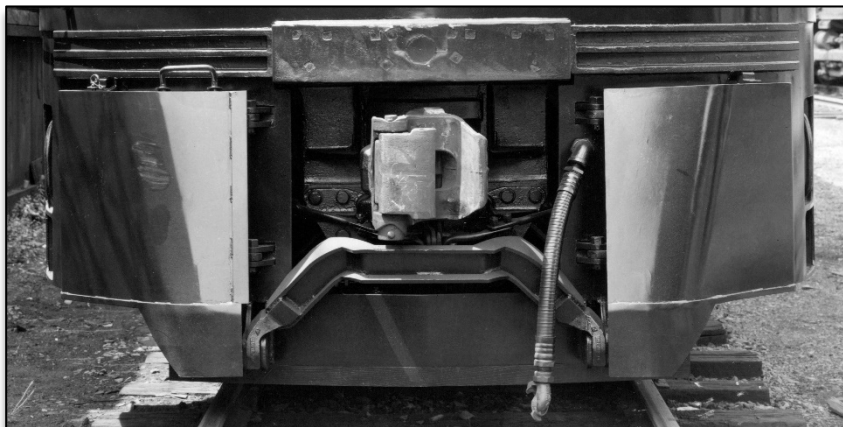
(Top) Close up of open coupler doors and pilot arch in up position on 9818A.
