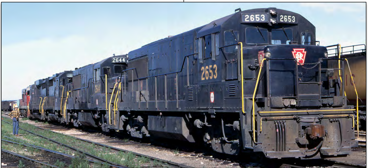
It is July 22, 1967 in Cheyenne, Wyoming and #2653 from the final order leads renumbered #2644, a GP35, a GP30, and a Burlington unit in run-through service. Note the two-piece windshield, cab roof radio antenna, radio sticker, and fuel filler and gauge in the center of the fuel tank. A UP gas turbine is to the right. (K. L. Douglas, William D. Volkmer collection)
