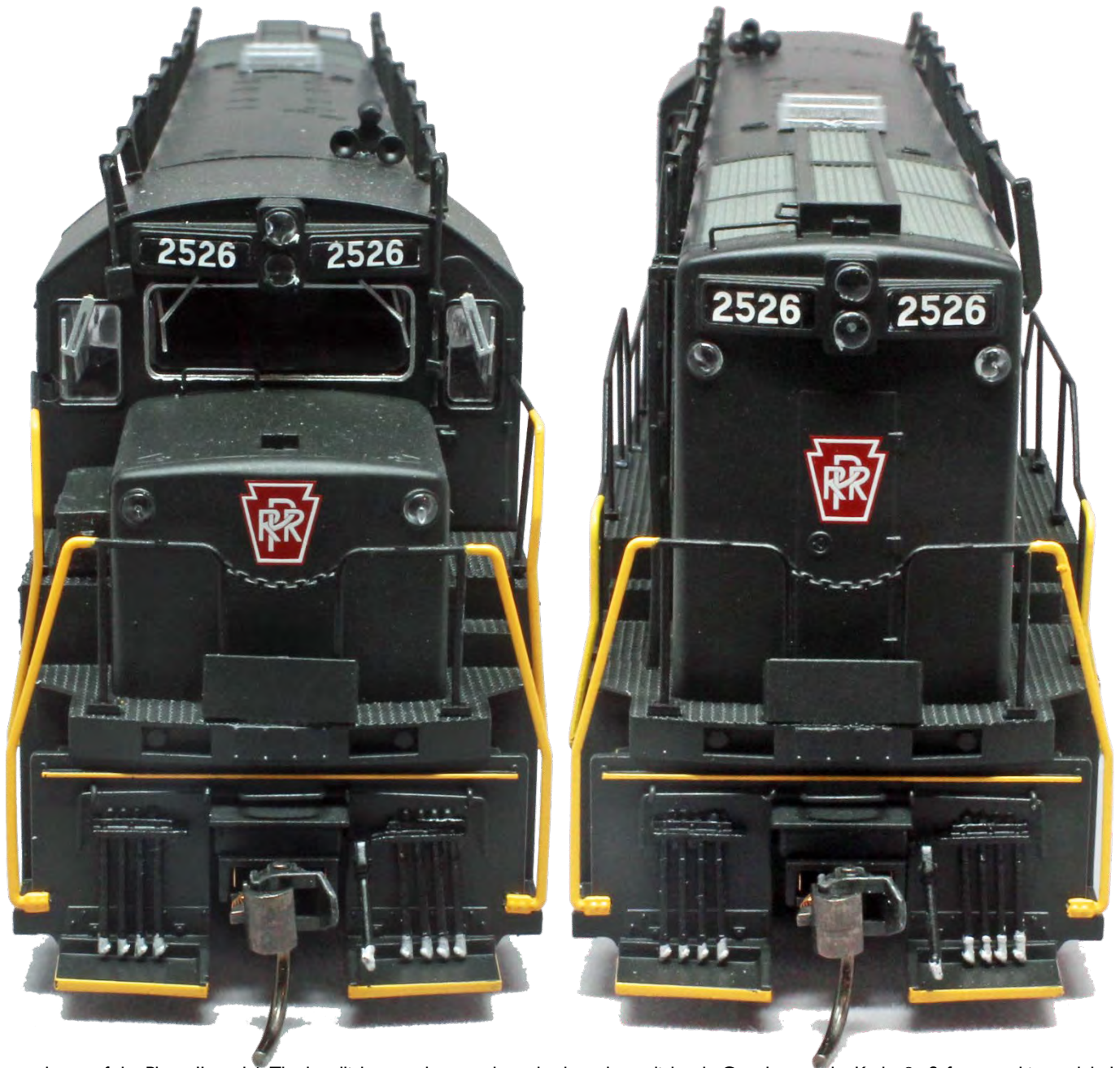
Front and rear of the Phase II model. The headlights, markers, and numberboards are lighted. Couplers are by Kadee®. Safety tread is modeled on the walkways. On the prototype, PRR painted the straight section of the cut lever above the MU hoses yellow for safety.
