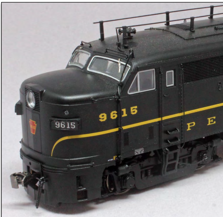
Stock FA2 nose section (pilot door piece not yet applied). Note the battery box door with vertical louvers correct for the early order group.
