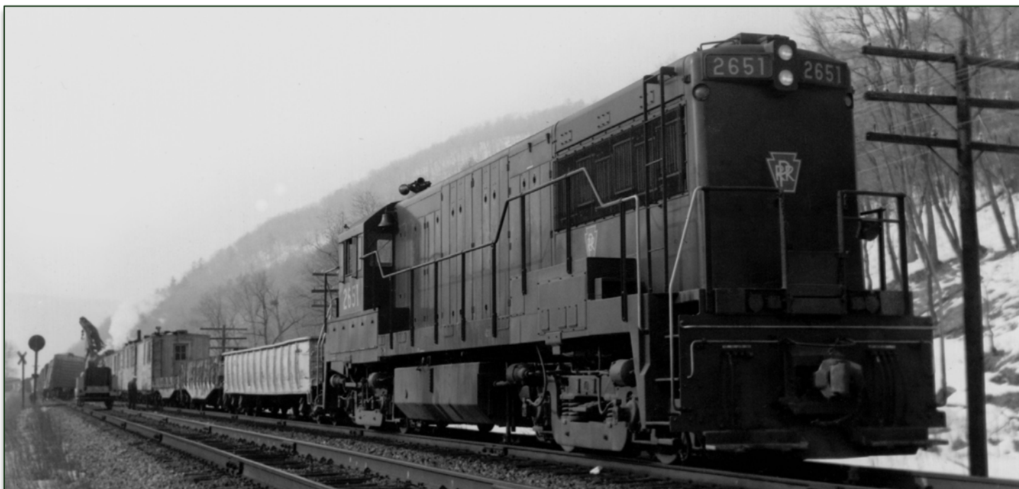
GF-25 #2651 is with the Northern Division wreck train in Lock Haven, Pa. (MP 212) on February 9, 1966. Dual controls would have been handy on this day, but this unit is from the final order and does not have them. Note the factory-installed ladder for access to the sand hatches. This is a Phase IV unit from the last order. The handrail stanchions are mounted on the outside of the frame. (William D. Volkmer)
