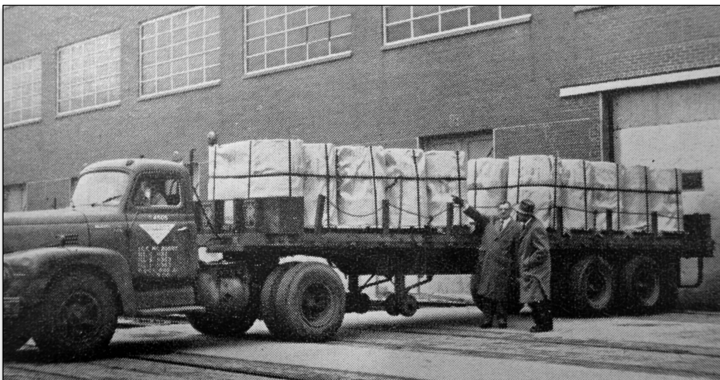
▲ View showing rear tailgate with placement of tailgate reinforcements, step bumper, and lettering placement. (PRR) ▼ Tandem axle trailer showing side stakes in place. This trailer appears to have a rectangular bulkhead in place of a round one. Trailer number unknown. (PRR)
