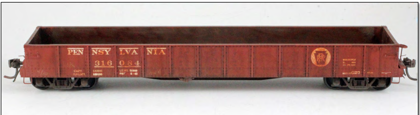
(Above and next page) The car was completed with scale couplers, Andrews style trucks, air hoses, and Carmer uncoupling levers and then it was painted, lettered and weathered.
