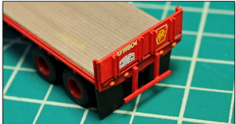
View shows lettering arrangement on tailgate, placement of rear tailgate reinforcements, and rear step bumper.
