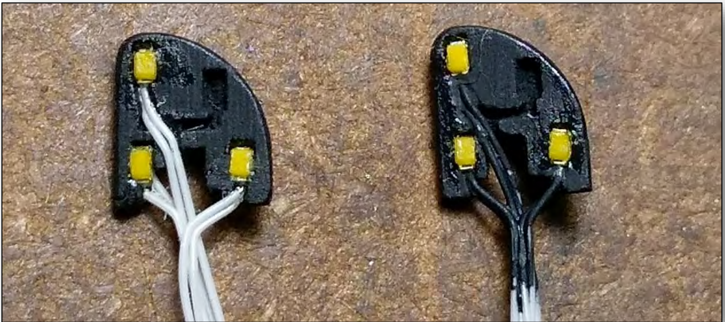
Two-aspect S-410-B drawers with LED's mounted and wires gathered and then painted, ready for assembly into housing.
