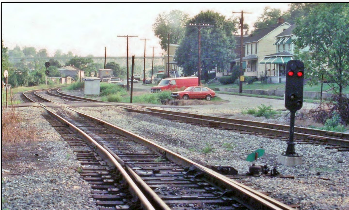
▲ Looking northward from the south end of the wye at West Brownsville Junction on the former Monongahela Division on 4/21/91. The southward main track at left is controlled by the dual-arm high home signal, however, the south leg of the wye converging from the right is the slow speed leg and joins the yard lead and thus only rates a low home signal. Since this diverging (converging) track ends behind the photo and thus requires a two-arm signal, a 2-aspect Pedestal type was used here. Note the wiring and lamp components are contained within the three locked compartments on its rear side. ▼ View southward from the same spot on 9/4/83. The northward high dual-arm home signal at the far end of "BROWN" interlocking can be seen in the distance beyond where the tracks converge. Like the high home signals, Pedestals also received "red eyes" on the upper arms later in the PRR era, this one displaying its STOP-SIGNAL aspect.
