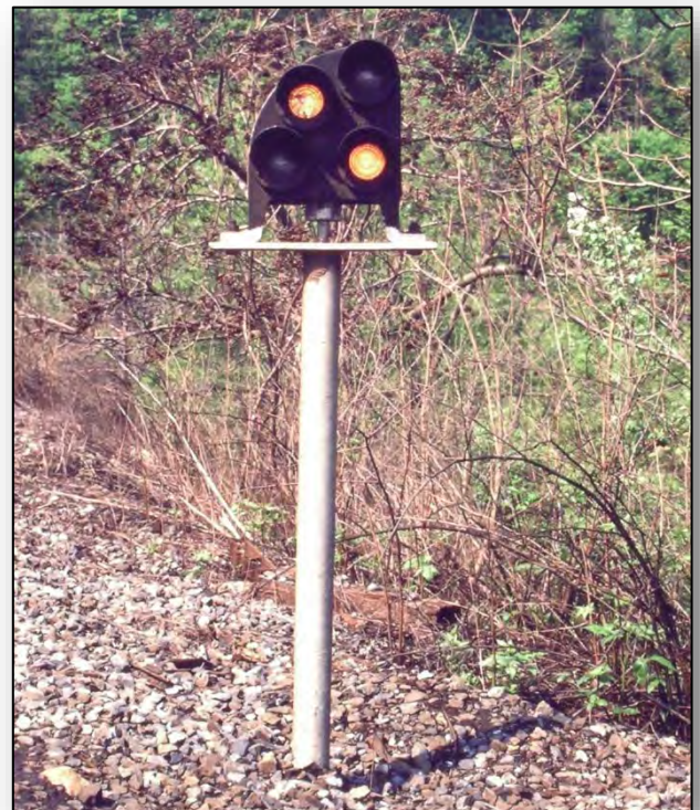
A dwarf, illustrating a special mounting on a short mast to provide adequate visibility based on the local conditions, displays RESTRICTING at the west end of the Rockville Bridge, 5/20/84.
