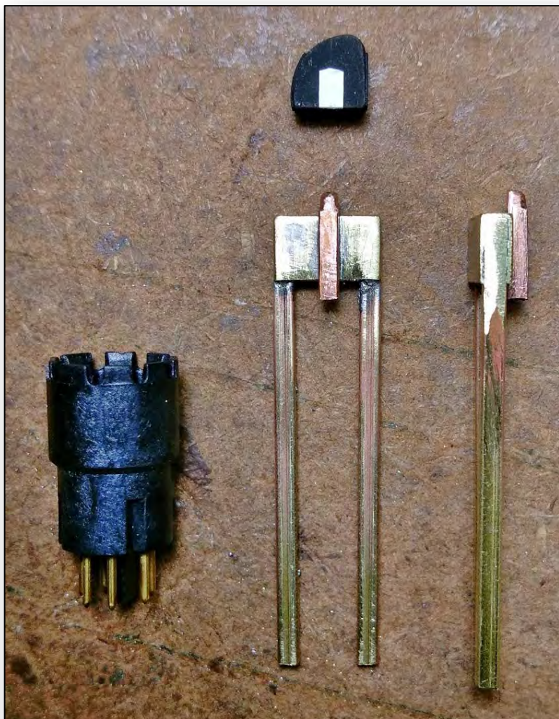
S-410-B mounting parts at left with simulated conduit soldered to foundation and raised piece added to back of signal housing. At right foundation assembly showing wire routing hole adjacent to conduit and foot pieces glued in place.
