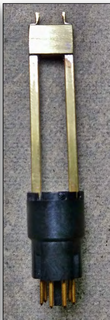
Individual parts for creating S-410-D foundation and mounting at left, soldered together at center with signal housing held in place to show proper leg spacing and base soldered into 6-pin Mini-Din plug connector at right.
