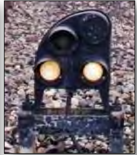
Typical mountings of S-410-D signals: a 4-aspect version displaying SLOW-CLEAR on a concrete foundation at left and at center, one displaying STOP-SIGNAL on a fabricated metal foundation at Northumberland. A 2-aspect signal also on a metal foundation displays STOP-SIGNAL. A former Signal Department employee related that they referred to these as "dumb" Dwarfs, since they could only display STOP-SIGNAL and RESTRICTING, i.e., stop or go (slowly). The three- or four-aspect Dwarfs gave more information on what was ahead.
