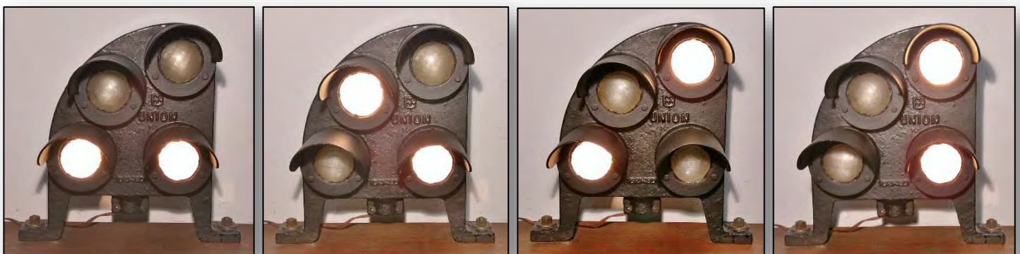
Preserved S-410-D displaying all four possible aspects: 1,4,5,7. From left to right: STOP-SIGNAL, RESTRICTING, SLOW-APPROACH, and SLOW-CLEAR. Note how white the light appears when the lenses are clean.
