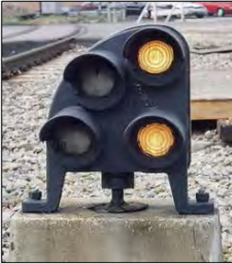
Typical mountings of S-410-D signals: a 4-aspect version displaying SLOW-CLEAR on a concrete foundation at left and at center, one displaying STOP-SIGNAL on a fabricated metal foundation at Northumberland. A 2-aspect signal also on a metal foundation displays STOP-SIGNAL. A former Signal Department employee related that they referred to these as "dumb" Dwarfs, since they could only display STOP-SIGNAL and RESTRICTING, i.e., stop or go (slowly). The three- or four-aspect Dwarfs gave more information on what was ahead.
